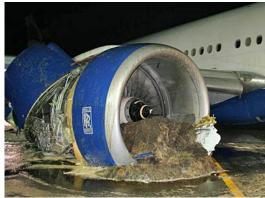
The evidence to date indicates that both engines had low fuel pressure at the inlet to the HP pump. Restrictions in the fuel system between the aircraft fuel tanks and each of the engine HP pumps, resulting in reduced fuel flows, is suspected." (AAIB)
